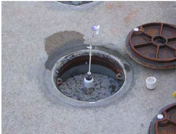
Figure 3.5.7.1 Soil Gas Sample Point with Sampling Apparatus Attached.
