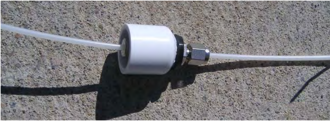
Figure 3.5.7.2 Cap Used for Soil Gas and Well Headspace Sampling.
