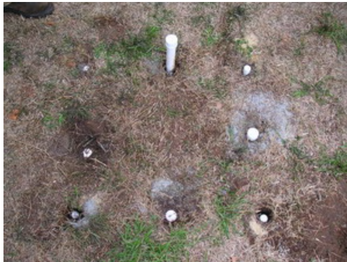
Figure 3.5.1.1: Soil Gas and Monitoring Well Cluster Prior to Pad Completion (Altus AFB).
